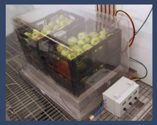
'Pods' in the room contain several bushels of apple Valves in the base open to admit room air Then close to allow the  $O_2$  and  $CO_2$  to change. RQ is measured and used to set lower  $O_2$  level
